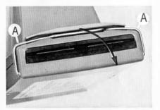
2. Unlock and open the back: Push up both ends of the back lock (A) and open the back all the way. Be careful not to drop the camera as the back opens.
