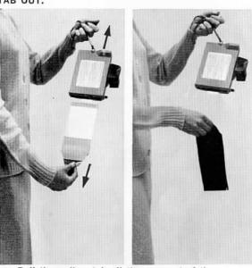
4. Pull the yellow tab all the way out of the camera: Pull it straight, smoothly, at medium speed, without slowing down or stopping.
