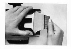
2. Without moving the pack, gently pull the yellow tab all the way out of the camera and discard that piece of film. Don't try to save it.
