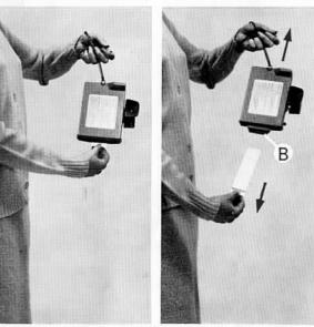
2. Pull the white tab (A) all the way out of the camera: This causes a yellow tab (B) to pop out of a narrow door in the end of the camera.
