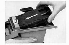
3. Insert the pack: Hold the film pack by the edges as shown. Push the closed end of the pack under the light shield (B) against a spring and then push the pack down into the camera.
