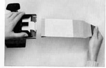
4. Close and lock the camera back, making sure that the next white tab (A) is outside and behind the lock (B), as shown.
